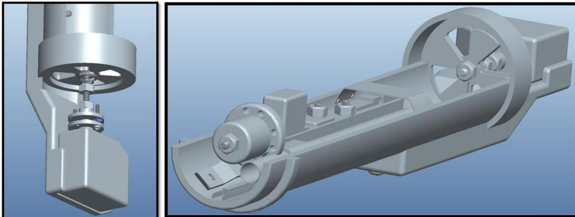
**Figure 1.** Zero-Pressure Valve System 3-D Model. Shown with Main Tube halved, to display internal components.
