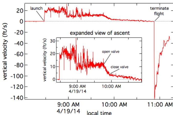
Figure 3. Vertical velocity profile for the BOREALIS 4/19/2014 Flight
